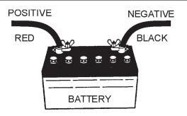
**Figure 34. Battery Connections**
